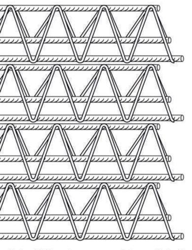
Electrowelded armatures are a product assembled with wires designed with a triangular structure. Their contact points are joined with electric welds.
