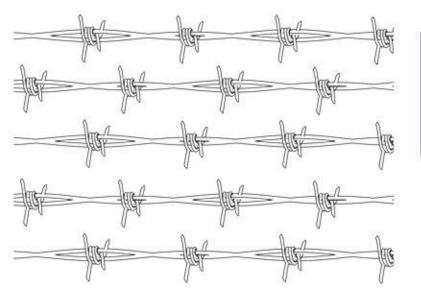
Magnacero's barbed wired is made with two galvanized wires threaded longitudinally and tied with two additional twisted wires that shape the barbs.
